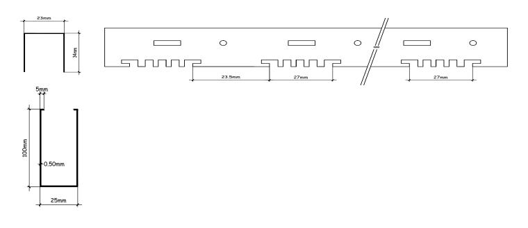
Baffle ceiling Fixing Detail
